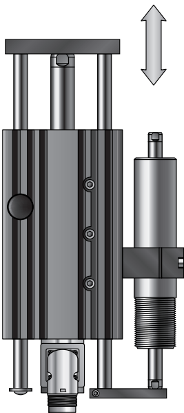
Weight compensation with MagSpring mounted on the side
