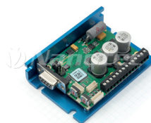
Controller SMCI36, 6A/24-72 V, fully programmable, for BLDC and stepper motors, dspDrive ® , Closed Loop, CANopen
