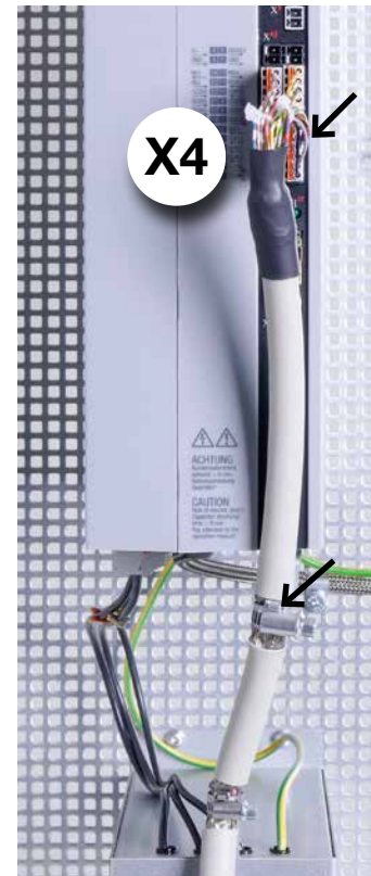
Figure 4.13 Specimen setup - detail 4: Control cables BG5
