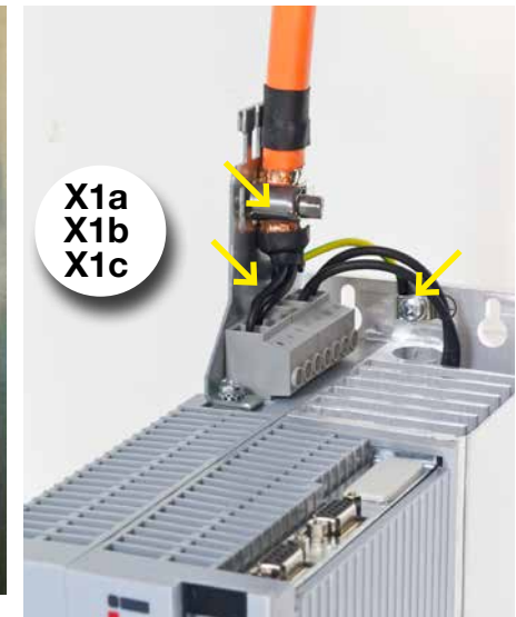
Figure 4.9 Detail 1: Motor cable BG5
