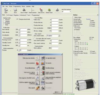
MacTalk software is the main interface for setting up the QuickStep motor for a specific application.
