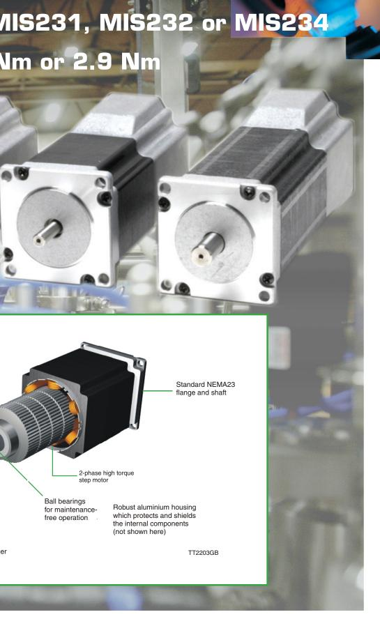
QuickStep is a new series of motors from JVL which can be delivered with a large selection of functions and in a wide variety of combinations. The base is a high-torque NEMA23 step motor with a housing so that IP55 or greater protection can be achieved. One or more circuit cards and different connectors can be mounted in the housing to adapt the motor to a given task.
