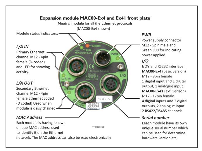
The standard expansion module MAC00-Ex4 is equipped with 1 analogue input, 1 digital input and 1 digital output. With the extended I/O version MAC00-Ex41, is used a 17 pin
