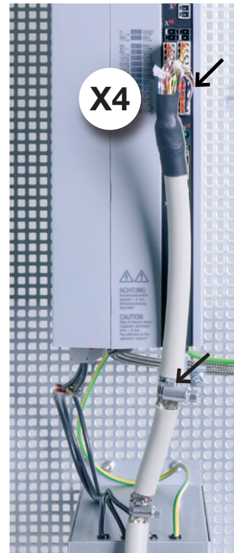
Figure 4.13 Specimen setup - detail 4: Control cables BG5
