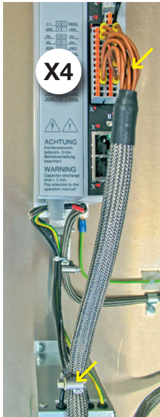
Figure 4.12 Specimen setup - detail 4: Control cables BG2 to BG4
