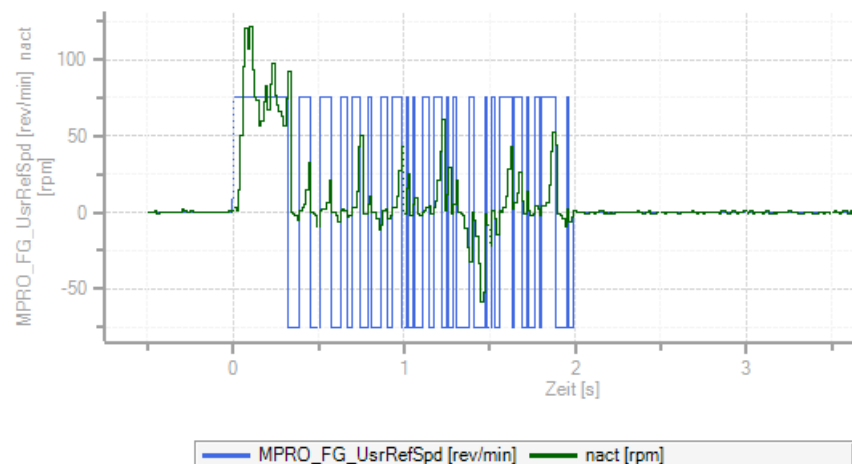
Fig. 8.34: PRBS-Signal: Amplitude = 150 rpm, Time = 20 ms
