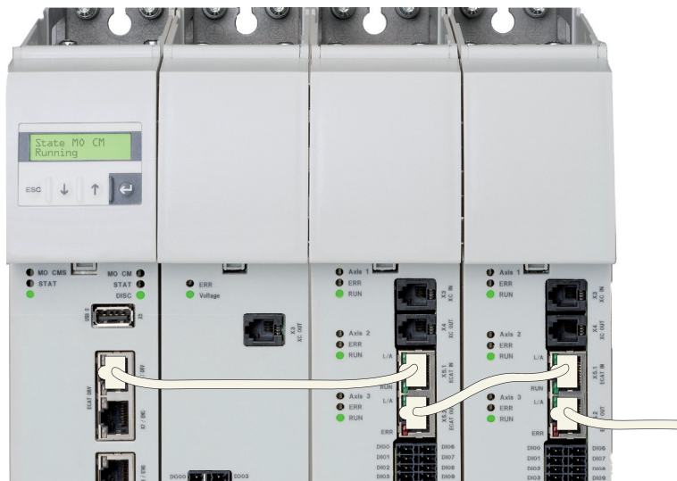
Figure 5.9 Connection of EtherCAT master with axis controller
