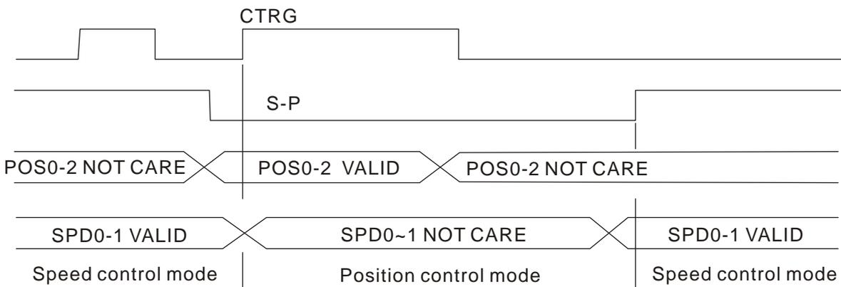
Figure 1. : Speed / Position Control Mode Selection
