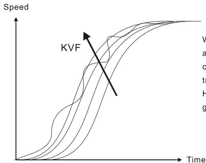
When the value of KVF is nearly to 1 and the forward compensation is more complete, then the value of dynamic tracking error will become very small. However, when the value of KVF is too great, it may cause vibration.
