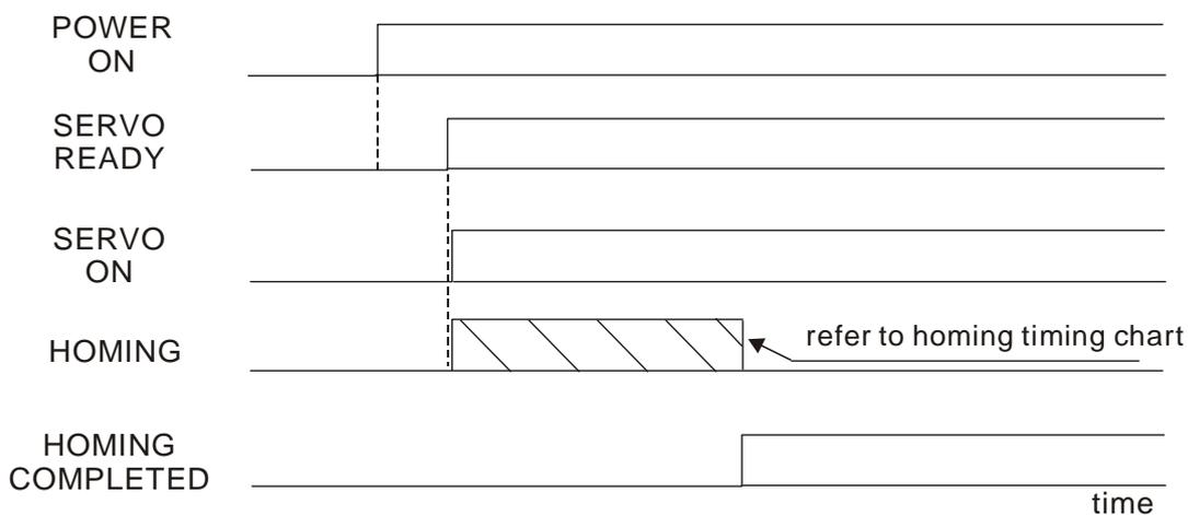
2. Enable homing function by input contact (SHOM) (C=2)
