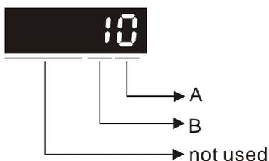
Monitor analog output polarity
