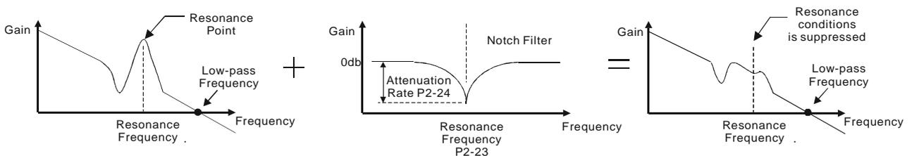
**Use Low-pass Filter to suppress resonance**
