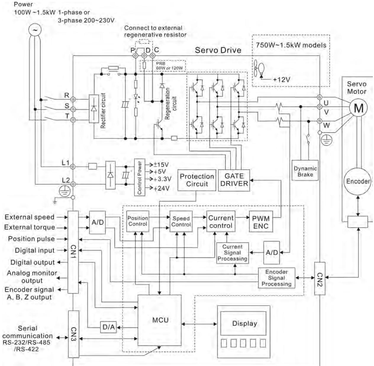
Figure 3.7 Basic Wiring Schematic of 2kW, 220V models
