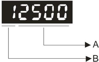
A: Range of the pulse numbers of encoder outputs
