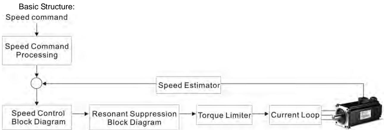
In the figure above, the speed command processing is used to select the command source of speed control according to chapter 6.3.1, including proportional gain (P1-40) and S-curve filter smoothing strategy of speed control. The speed control block diagram is used to manage the gain parameters of the servo drive and calculate the current input provided to motor instantaneously. The resonance suppression block diagram is used to suppress the resonance of mechanical system.
