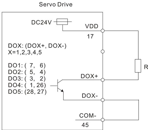
**C6: Wiring of DO signal, for the use of internal power supply, inductive load**
