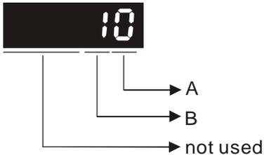
A: Monitor analog output polarity
