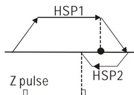
**P1 - 49****HSPD2 2nd Speed Setting of Low Speed Homing****Communication Addr.: 0131H**
