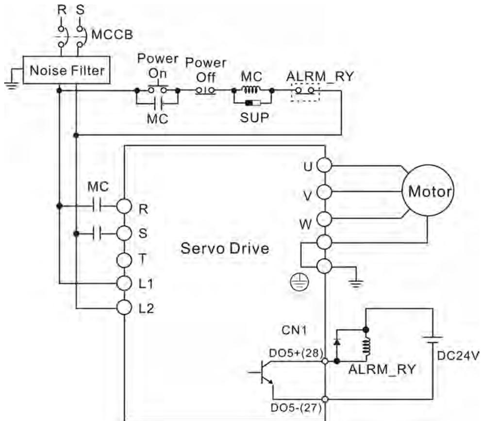
Figure 3.4 Single-Phase Power Supply (400W and below, 110V models)
