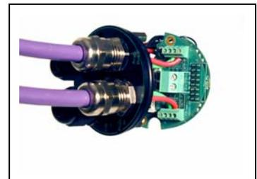
Attach the circuit board to the rear plate with the two screws. **REMEMBER** to use the spring washers included.
