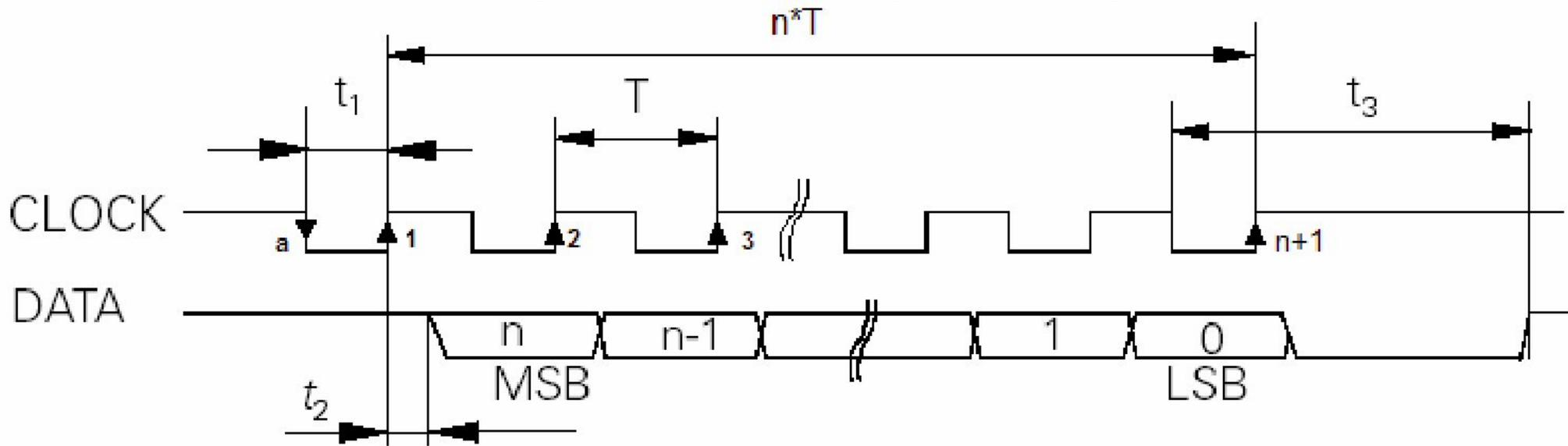
Figure 1 – Typical SSI Timing Diagram
