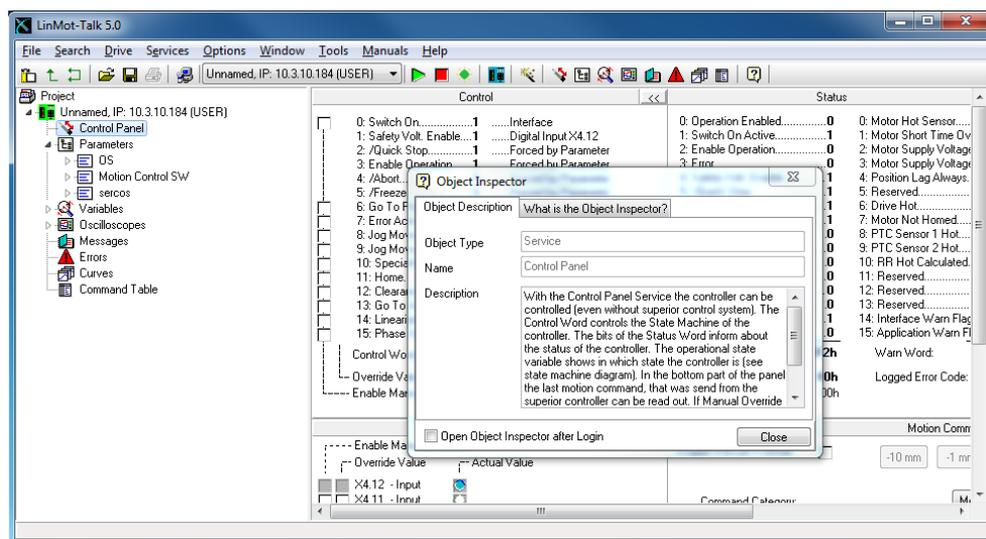
The Object Inspector window can be dragged away or closed. It can be reopened with F1.
