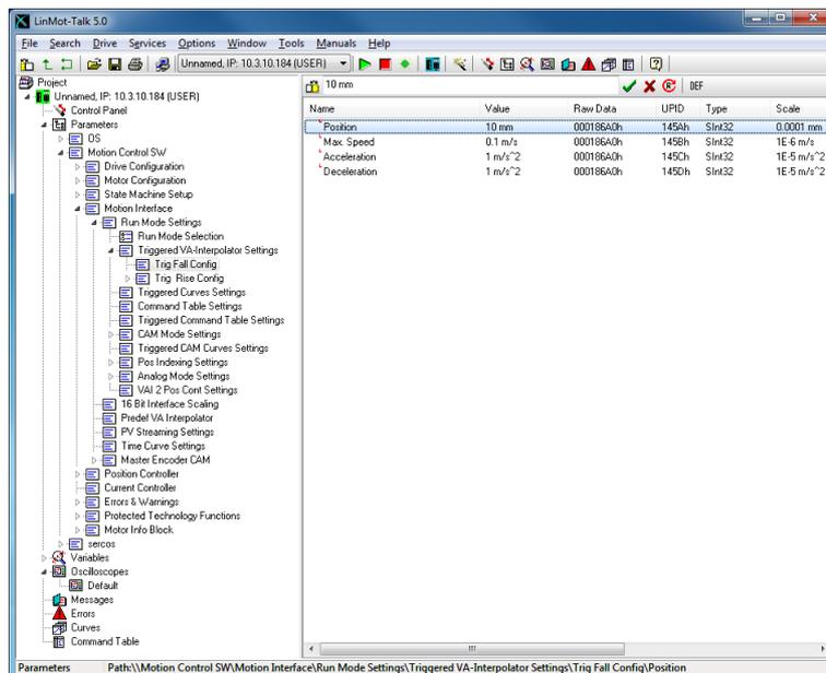
This is all we have to configure. The speed, acceleration and deceleration can also be defined at this place in the parameter tree. The motor can now be started the same way as described under 3.17 Control Status.
