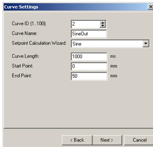
In this mask, we will set the curve ID to 2 (we will have the merged curve with ID 1 at the end) and as name we set e.g. “SineOut”. The end point is placed at 50mm. With “Next” the wizard will show some curve data:
