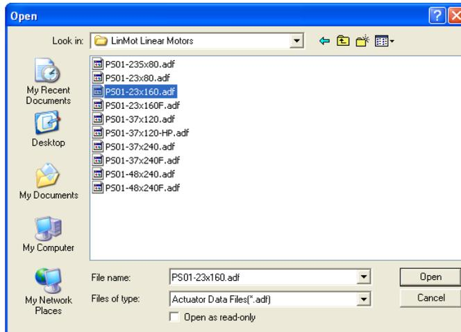
Select the actuator type you have wired to the drive, then press Open. The following steps will show forms including drawings and descriptive texts. The first step is to define the stator and slider.
