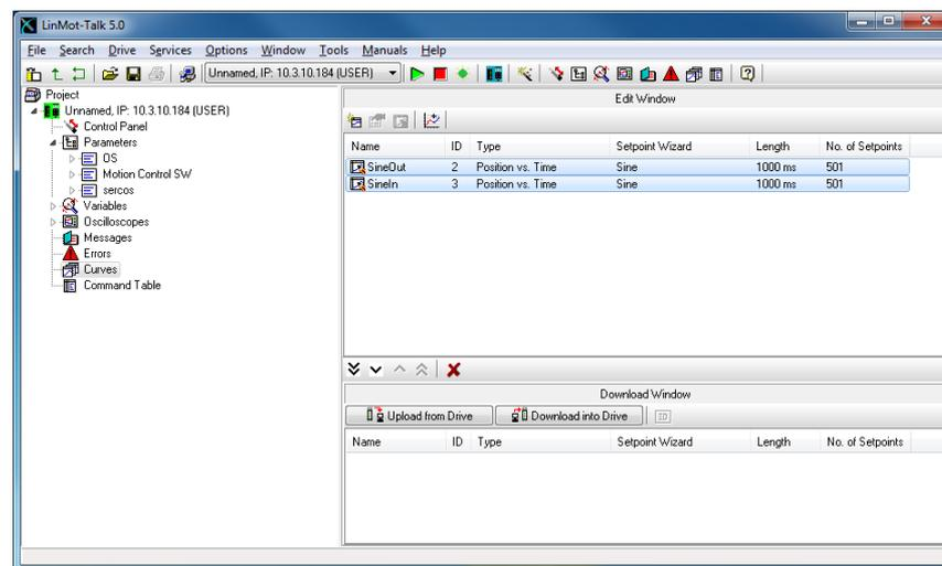
then press the “Join Curves” button
