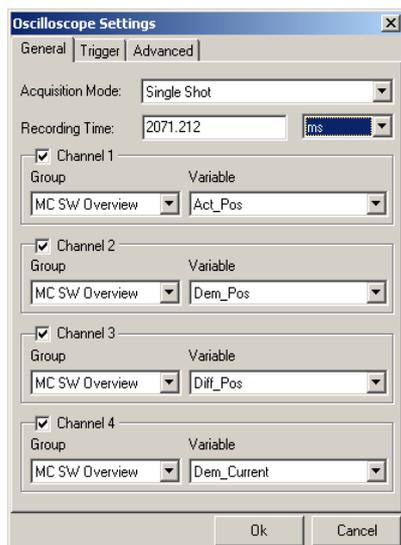
Then press Ok and start the oscilloscope with
