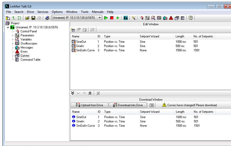
The curve tool is divided into the edit and the download window. The edit window is used to generate, merge and modify curves with the following buttons:
