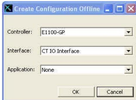
The above window will be shown. Select the drive first, then choose the interface and application software. The software parts, which can be selected, are the same as when installing firmware to the drive. When created the configuration, the parameters will have their default values. The configuration can then be altered and saved the normal way.
