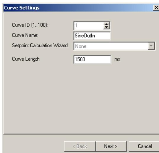
We will set the curve name to “SineOutIn” and make sure the curve ID is 1. The curve length is proposed as the sum of the curve segment times. Press “Next” and “Finish”. The curve for the continuous curve mode is now defined and has, according to the parameter settings, the curve ID 1. As we want to download the curves to the drive we select all the curves in the edit window and move them to the download window.
