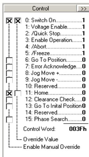
Now turn off and turn on again the “Switch On” flag, this is because of the auto start prevention. At this time, the motor will be powered and position controlled at the actual position. Set the “Home” flag and the motor will initialize against the inner hard stop. When the motor stands still, clear the “Home” flag and the motor will run the curve continuously.
