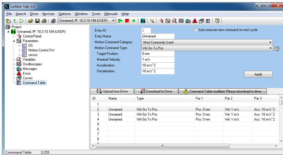
A big variety of commands can be set in this tables, such as motion commands, conditions, sequence directives, parameter access, ... This makes the CT to very powerful functional unit. The CT entries can be accessed (executed) via digital inputs (on X6) or via interface software. The CT tool has the following editing elements:
