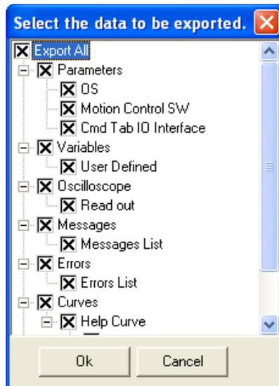
It is recommended to export all. For a configuration recovery it is necessary to select the parameters, curves and command table.
