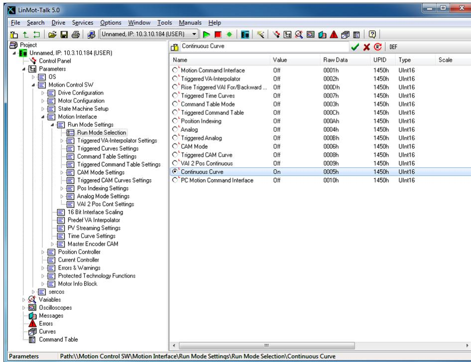
The second parameter to be set is to define which curve has to be run. Set the parameter “Curve ID” to 1 under \Motion Control SW\Motion Interface\Time Curve Settings\.
