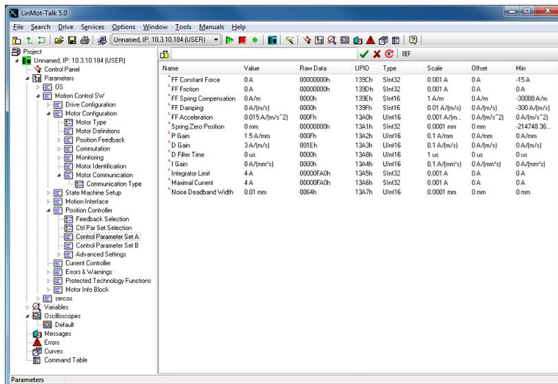
Parameters, which are marked as live (
