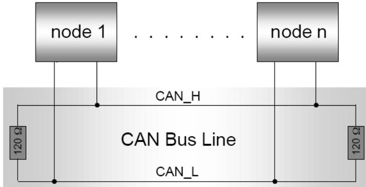
For easy installation, the LinMot DeviceNet drives have built in termination resistors, which can be activated, if the LinMot drive is at the end of the bus line, and if there is no termination in the connector.
