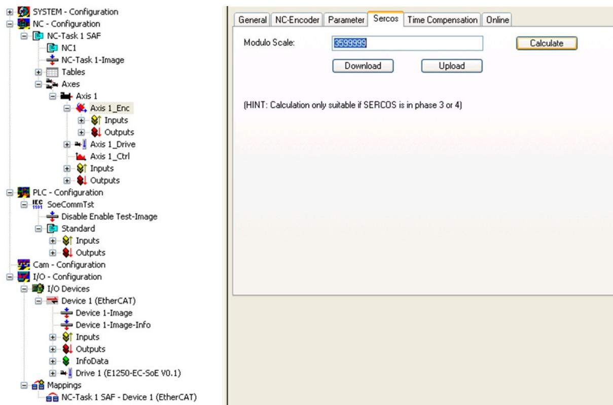
Now the NC encoder has to be set to the correct value push the calculate button for this reason.
