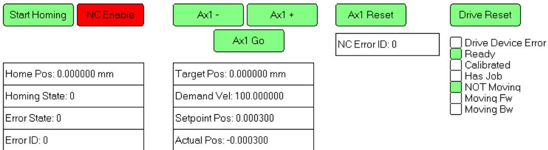
Push the homing button is released when finished now “Calibrated” should be highlighted:
