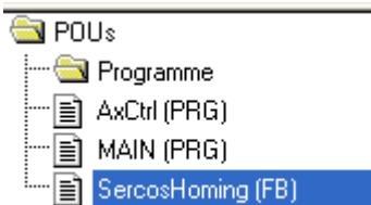
In the FB SercosHoming the drive based homing is done. The AxCtrl program handles the user inputs of the HOMING\_PANEL visualization.
