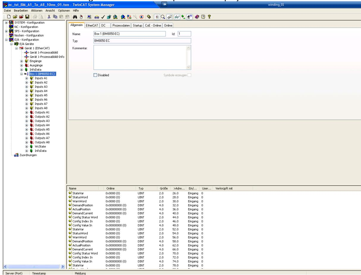
In this example the scan found a BM8050-EC bus module, which is imported to the project. The bus module has IO data for 8 Axis configured by default. If less than 8 Axis are needed some axis can be deleted (see chapter 5).
