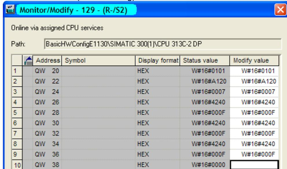
In the case of \Parameters\PROFINET Interface\Byte/Word Order\MC CMD Intf Par Order\ reversed:
