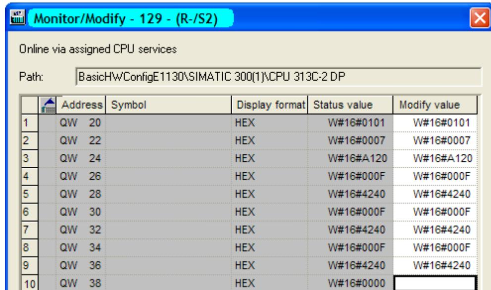
To send the next command the count nibble has to be changed. The header for the next VAI Go To Pos command is therefore 0100h.
