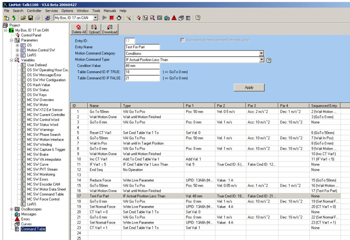
The first sequence ID1, ID2 and ID3 shows a simple sequence GoTo 50mm wait until motion is completed and then go back to 0mm.
