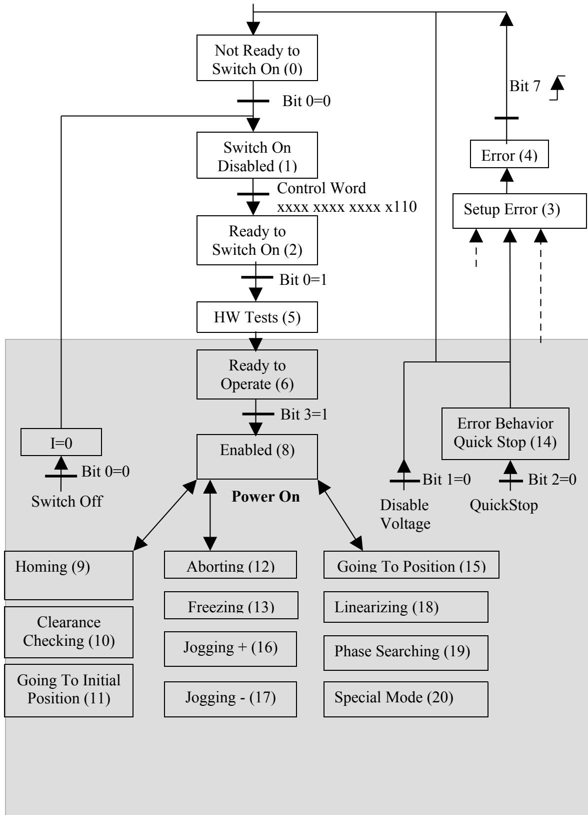
The state machine can be followed in the PLCs with fieldbus using the StateVar. This response word can be configured for any supported fieldbus.
