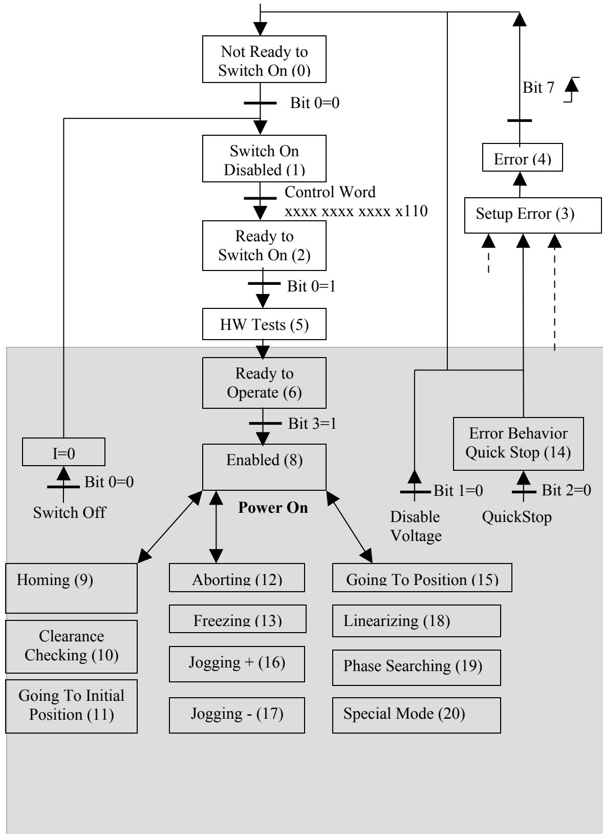
The state machine can be followed in the PLCs with fieldbus using the StateVar. This response word can be configured for any supported fieldbus.
