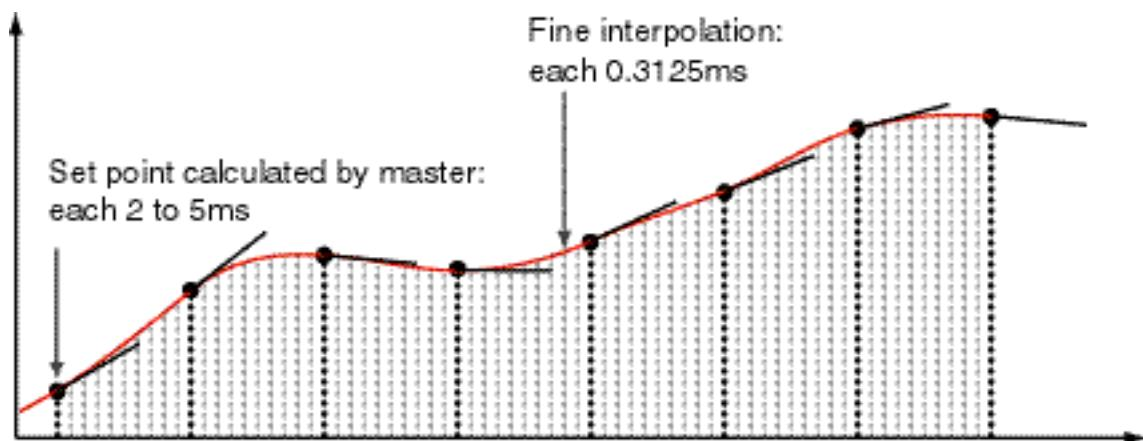
In the P- streaming mode, it is possible that, depending on the cycle time, a quiet noisy motion is generated, this because of the twice derivation of the position signal to generate the acceleration value. In this case, it is recommended to set the position controller value "FF Acceleration" (UPID 0x13A0 and 0x13B4) to zero.
