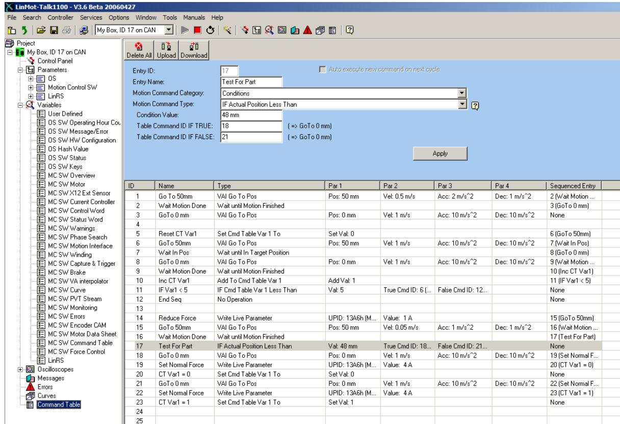
The first sequence ID1, ID2 and ID3 shows a simple sequence GoTo 50mm wait until motion is completed and then go back to 0mm.
