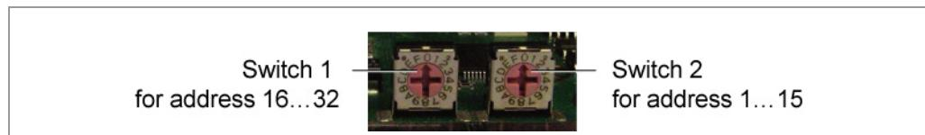
The 16's place is set with switch 1 (left) and the 1's place is set with switch 2 (right).
