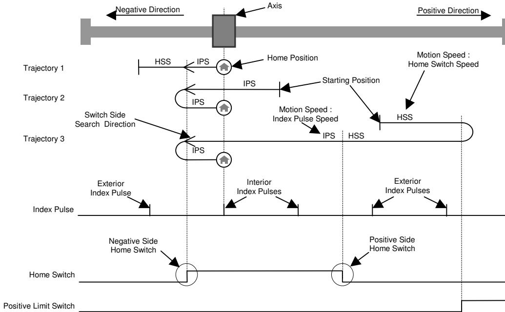
For simplifying diagrams, the trajectory of the switch side search is not explicitly drawn. However, an arrow indicates the direction used to search a switch side. Hence, trajectory 1 of homing method 8 is explained in the following diagram:
