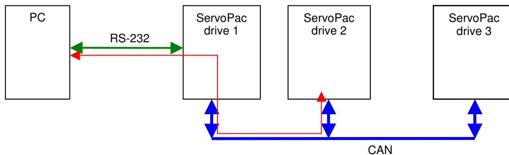
The ServoPac drive supports Node ID setting by switches from 1 to 63.
