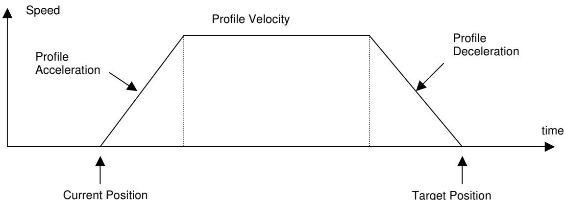
In profile position mode, these bits in the control word are relative to the control of the trajectory:
