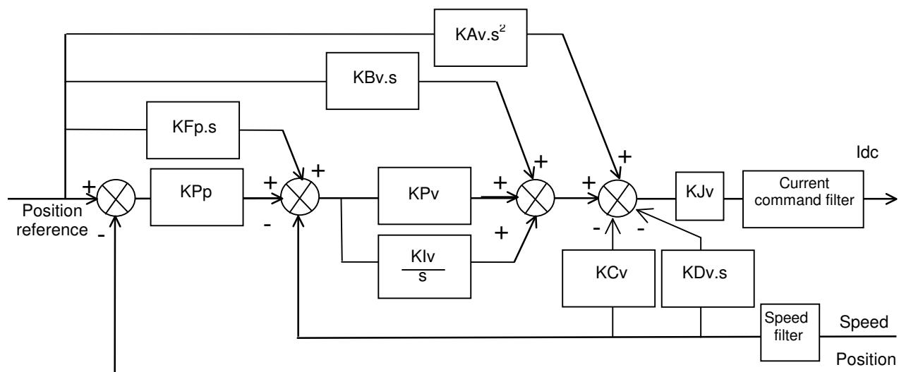
**Speed loop** gains are the most critical adjust because they greatly depend on the mechanical load characteristics (inertias, frictions, coupling stiffness, resonances,...).
