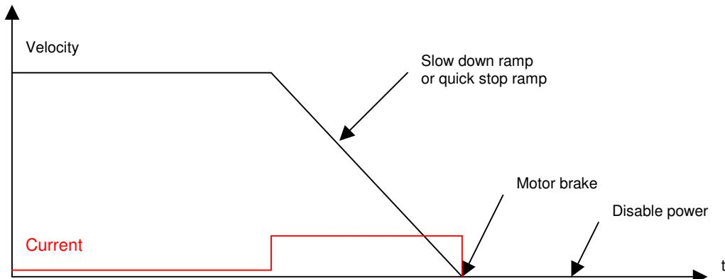
With stop on current limit, the motor is slowed down in velocity loop with a current limitation.
