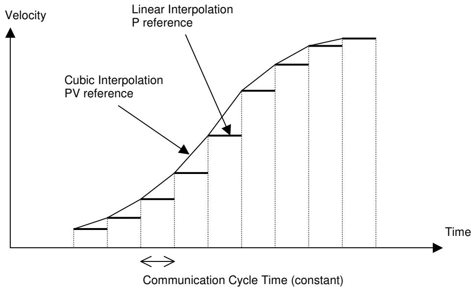
Note: The velocity reference for each set-point must be the instantaneous velocity at this point (not the average velocity).
