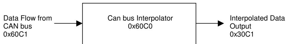
The CAN bus Interpolator is running in any mode but the result of the interpolator (0x30C1) is applied to the position loop only in Interpolated Position Mode.
