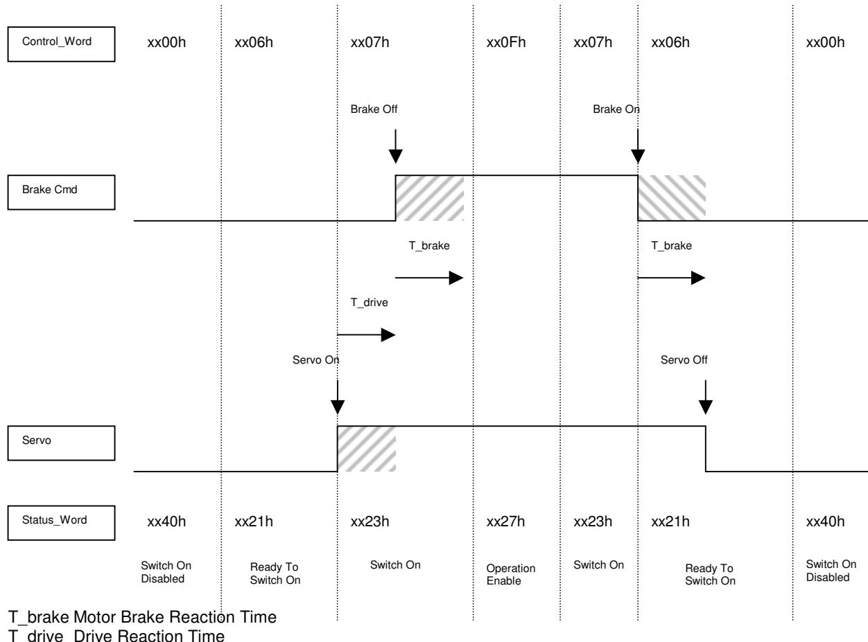
**Note:** The motor brake control is automatic with Switch On/Off by the control\_word. To disable the motor brake control, it is necessary to set at 1 bit 0 of object 60FE sub-index 2 (digital output bitmask). The motor brake is then manually controlled by bit 0 of object 60FE sub-index 1.
