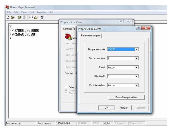
After change to a remote node, RD and WR are applied to this remote node.
